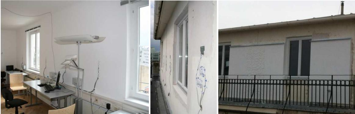
Fig. 1. Position of the temperature and humidity sensors (a) internal surface; (b) external surface prior to retrofit; (c) on the F222 plaster beneath the finish (not visible) after retrofit
